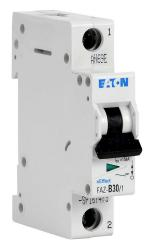
Eaton miniature supplementary protector, 30A, 277 VAC / 48 VDC, 1-pole, B curve, thermal magnetic, 10kA @ 277 VAC interrupting rating, 35mm DIN rail mount.
