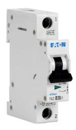
Eaton miniature supplementary protector, 30A, 277 VAC / 48 VDC, 1-pole, B curve, thermal magnetic, 10kA @ 277 VAC interrupting rating, 35mm DIN rail mount.
