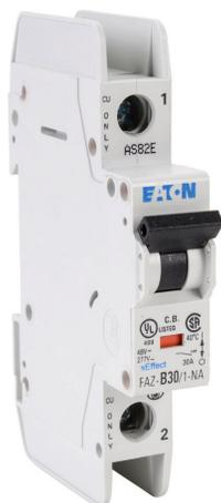
Eaton miniature circuit breaker, current-limiting, 30A, 277 VAC / 48 VDC, 1-pole, B curve, thermal magnetic, 10kA @ 277 VAC interrupting rating, 35mm DIN rail mount.
