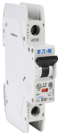
Eaton miniature circuit breaker, current-limiting, 30A, 240 VAC / 48 VDC, 1-pole, B curve, thermal magnetic, 10kA @ 240 VAC interrupting rating, 35mm DIN rail mount.
