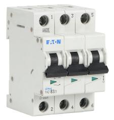
Eaton miniature supplementary protector, 3A, 480Y / 277 VAC / 96 VDC, 3-pole, B curve, thermal magnetic, 10kA @ 480Y/277 VAC interrupting rating, 35mm DIN rail mount.
