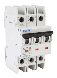
Eaton miniature circuit breaker, current-limiting, 3A, 480Y / 277 VAC / 96 VDC, 3-pole, B curve, thermal magnetic, 10kA @ 480Y/277 VAC interrupting rating, 35mm DIN rail mount.
