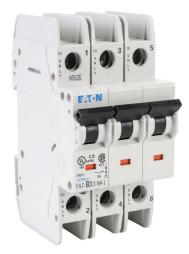
Eaton miniature circuit breaker, current-limiting, 3A, 240 VAC / 96 VDC, 3-pole, B curve, thermal magnetic, 10kA @ 240 VAC interrupting rating, 35mm DIN rail mount.
