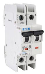
Eaton miniature circuit breaker, current-limiting, 3A, 480Y / 277 VAC / 96 VDC, 2-pole, B curve, thermal magnetic, 10kA @ 480Y/277 VAC interrupting rating, 35mm DIN rail mount.
