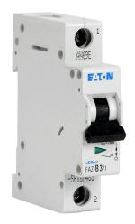
Eaton miniature supplementary protector, 3A, 277 VAC / 48 VDC, 1-pole, B curve, thermal magnetic, 10kA @ 277 VAC interrupting rating, 35mm DIN rail mount.
