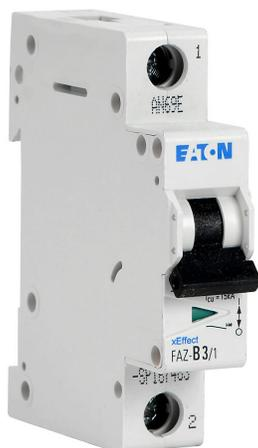
Eaton miniature supplementary protector, 3A, 277 VAC / 48 VDC, 1-pole, B curve, thermal magnetic, 10kA @ 277 VAC interrupting rating, 35mm DIN rail mount.
