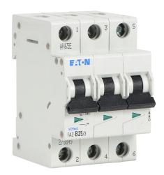
Eaton miniature supplementary protector, 25A, 480Y / 277 VAC / 96 VDC, 3-pole, B curve, thermal magnetic, 10kA @ 480Y/277 VAC interrupting rating, 35mm DIN rail mount.
