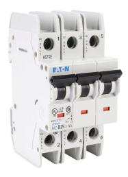
Eaton miniature circuit breaker, current-limiting, 25A, 480Y / 277 VAC / 96 VDC, 3-pole, B curve, thermal magnetic, 14kA @ 480Y/277 VAC interrupting rating, 35mm DIN rail mount.
