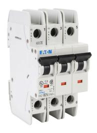
Eaton miniature circuit breaker, current-limiting, 25A, 240 VAC / 96 VDC, 3-pole, B curve, thermal magnetic, 14kA @ 240 VAC interrupting rating, 35mm DIN rail mount.
