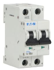
Eaton miniature supplementary protector, 25A, 480Y / 277 VAC / 96 VDC, 2-pole, B curve, thermal magnetic, 10kA @ 480Y/277 VAC interrupting rating, 35mm DIN rail mount.
