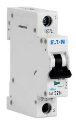
Eaton miniature supplementary protector, 25A, 277 VAC / 48 VDC, 1-pole, B curve, thermal magnetic, 10kA @ 277 VAC interrupting rating, 35mm DIN rail mount.
