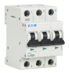
Eaton miniature supplementary protector, 20A, 480Y / 277 VAC / 96 VDC, 3-pole, B curve, thermal magnetic, 10kA @ 480Y/277 VAC interrupting rating, 35mm DIN rail mount.
