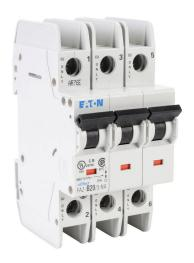
Eaton miniature circuit breaker, current-limiting, 20A, 480Y / 277 VAC / 96 VDC, 3-pole, B curve, thermal magnetic, 14kA @ 480Y/277 VAC interrupting rating, 35mm DIN rail mount.
