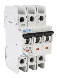
Eaton miniature circuit breaker, current-limiting, 20A, 240 VAC / 96 VDC, 3-pole, B curve, thermal magnetic, 14kA @ 240 VAC interrupting rating, 35mm DIN rail mount.
