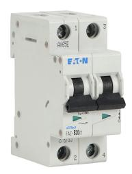
Eaton miniature supplementary protector, 20A, 480Y / 277 VAC / 96 VDC, 2-pole, B curve, thermal magnetic, 10kA @ 480Y/277 VAC interrupting rating, 35mm DIN rail mount.
