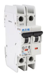
Eaton miniature circuit breaker, current-limiting, 20A, 240 VAC / 96 VDC, 2-pole, B curve, thermal magnetic, 14kA @ 240 VAC interrupting rating, 35mm DIN rail mount.
