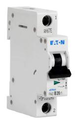
Eaton miniature supplementary protector, 20A, 277 VAC / 48 VDC, 1-pole, B curve, thermal magnetic, 10kA @ 277 VAC interrupting rating, 35mm DIN rail mount.
