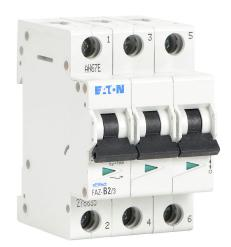
Eaton miniature supplementary protector, 2A, 480Y / 277 VAC / 96 VDC, 3-pole, B curve, thermal magnetic, 10kA @ 480Y/277 VAC interrupting rating, 35mm DIN rail mount.
