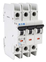
Eaton miniature circuit breaker, current-limiting, 2A, 480Y / 277 VAC / 96 VDC, 3-pole, B curve, thermal magnetic, 10kA @ 480Y/277 VAC interrupting rating, 35mm DIN rail mount.
