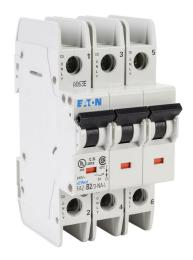
Eaton miniature circuit breaker, current-limiting, 2A, 240 VAC / 96 VDC, 3-pole, B curve, thermal magnetic, 10kA @ 240 VAC interrupting rating, 35mm DIN rail mount.
