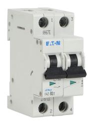
Eaton miniature supplementary protector, 2A, 480Y / 277 VAC / 96 VDC, 2-pole, B curve, thermal magnetic, 10kA @ 480Y/277 VAC interrupting rating, 35mm DIN rail mount.
