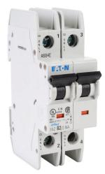
Eaton miniature circuit breaker, current-limiting, 2A, 480Y / 277 VAC / 96 VDC, 2-pole, B curve, thermal magnetic, 10kA @ 480Y/277 VAC interrupting rating, 35mm DIN rail mount.
