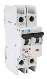
Eaton miniature circuit breaker, current-limiting, 2A, 240 VAC / 96 VDC, 2-pole, B curve, thermal magnetic, 10kA @ 240 VAC interrupting rating, 35mm DIN rail mount.
