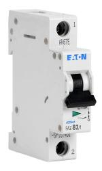
Eaton miniature supplementary protector, 2A, 277 VAC / 48 VDC, 1-pole, B curve, thermal magnetic, 10kA @ 277 VAC interrupting rating, 35mm DIN rail mount.
