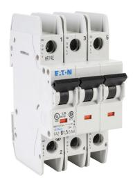
Eaton miniature circuit breaker, current-limiting, 1.5A, 480Y / 277 VAC / 96 VDC, 3-pole, B curve, thermal magnetic, 10kA @ 480Y/277 VAC interrupting rating, 35mm DIN rail mount.
