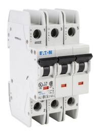
Eaton miniature circuit breaker, current-limiting, 1.5A, 240 VAC / 96 VDC, 3-pole, B curve, thermal magnetic, 10kA @ 240 VAC interrupting rating, 35mm DIN rail mount.
