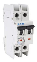
Eaton miniature circuit breaker, current-limiting, 1.5A, 240 VAC / 96 VDC, 2-pole, B curve, thermal magnetic, 10kA @ 240 VAC interrupting rating, 35mm DIN rail mount.
