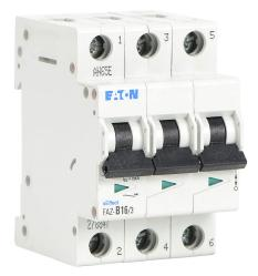
Eaton miniature supplementary protector, 16A, 480Y / 277 VAC / 96 VDC, 3-pole, B curve, thermal magnetic, 10kA @ 480Y/277 VAC interrupting rating, 35mm DIN rail mount.
