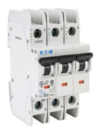
Eaton miniature circuit breaker, current-limiting, 16A, 240 VAC / 96 VDC, 3-pole, B curve, thermal magnetic, 14kA @ 240 VAC interrupting rating, 35mm DIN rail mount.
