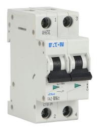
Eaton miniature supplementary protector, 16A, 480Y / 277 VAC / 96 VDC, 2-pole, B curve, thermal magnetic, 10kA @ 480Y/277 VAC interrupting rating, 35mm DIN rail mount.
