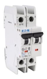
Eaton miniature circuit breaker, current-limiting, 16A, 480Y / 277 VAC / 96 VDC, 2-pole, B curve, thermal magnetic, 14kA @ 480Y/277 VAC interrupting rating, 35mm DIN rail mount.
