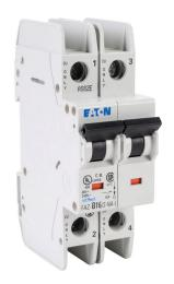
Eaton miniature circuit breaker, current-limiting, 16A, 240 VAC / 96 VDC, 2-pole, B curve, thermal magnetic, 14kA @ 240 VAC interrupting rating, 35mm DIN rail mount.
