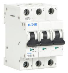
Eaton miniature supplementary protector, 15A, 480Y / 277 VAC / 96 VDC, 3-pole, B curve, thermal magnetic, 10kA @ 480Y/277 VAC interrupting rating, 35mm DIN rail mount.
