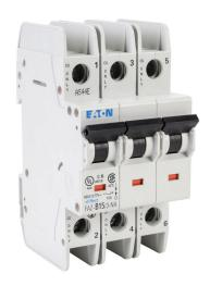
Eaton miniature circuit breaker, current-limiting, 15A, 480Y / 277 VAC / 96 VDC, 3-pole, B curve, thermal magnetic, 14kA @ 480Y/277 VAC interrupting rating, 35mm DIN rail mount.
