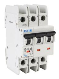
Eaton miniature circuit breaker, current-limiting, 15A, 240 VAC / 96 VDC, 3-pole, B curve, thermal magnetic, 14kA @ 240 VAC interrupting rating, 35mm DIN rail mount.
