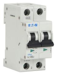
Eaton miniature supplementary protector, 15A, 480Y / 277 VAC / 96 VDC, 2-pole, B curve, thermal magnetic, 10kA @ 480Y/277 VAC interrupting rating, 35mm DIN rail mount.
