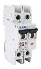
Eaton miniature circuit breaker, current-limiting, 15A, 480Y / 277 VAC / 96 VDC, 2-pole, B curve, thermal magnetic, 14kA @ 480Y/277 VAC interrupting rating, 35mm DIN rail mount.
