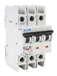
Eaton miniature circuit breaker, current-limiting, 13A, 240 VAC / 96 VDC, 3-pole, B curve, thermal magnetic, 10kA @ 240 VAC interrupting rating, 35mm DIN rail mount.
