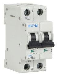
Eaton miniature supplementary protector, 13A, 480Y / 277 VAC / 96 VDC, 2-pole, B curve, thermal magnetic, 10kA @ 480Y/277 VAC interrupting rating, 35mm DIN rail mount.
