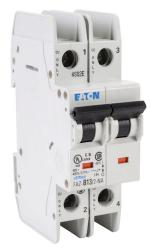
Eaton miniature circuit breaker, current-limiting, 13A, 480Y / 277 VAC / 96 VDC, 2-pole, B curve, thermal magnetic, 10kA @ 480Y/277 VAC interrupting rating, 35mm DIN rail mount.
