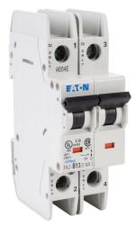
Eaton miniature circuit breaker, current-limiting, 13A, 240 VAC / 96 VDC, 2-pole, B curve, thermal magnetic, 10kA @ 240 VAC interrupting rating, 35mm DIN rail mount.
