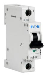
Eaton miniature supplementary protector, 13A, 277 VAC / 48 VDC, 1-pole, B curve, thermal magnetic, 10kA @ 277 VAC interrupting rating, 35mm DIN rail mount.
