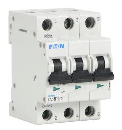
Eaton miniature supplementary protector, 10A, 480Y / 277 VAC / 96 VDC, 3-pole, B curve, thermal magnetic, 10kA @ 480Y/277 VAC interrupting rating, 35mm DIN rail mount.
