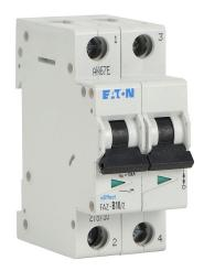
Eaton miniature supplementary protector, 10A, 480Y / 277 VAC / 96 VDC, 2-pole, B curve, thermal magnetic, 10kA @ 480Y/277 VAC interrupting rating, 35mm DIN rail mount.
