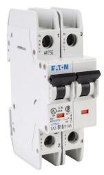
Eaton miniature circuit breaker, current-limiting, 10A, 480Y / 277 VAC / 96 VDC, 2-pole, B curve, thermal magnetic, 10kA @ 480Y/277 VAC interrupting rating, 35mm DIN rail mount.
