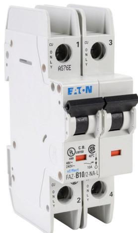
Eaton miniature circuit breaker, current-limiting, 10A, 240 VAC / 96 VDC, 2-pole, B curve, thermal magnetic, 10kA @ 240 VAC interrupting rating, 35mm DIN rail mount.
