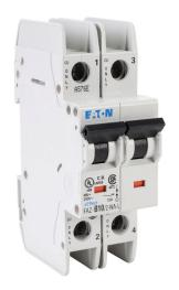
Eaton miniature circuit breaker, current-limiting, 10A, 240 VAC / 96 VDC, 2-pole, B curve, thermal magnetic, 10kA @ 240 VAC interrupting rating, 35mm DIN rail mount.
