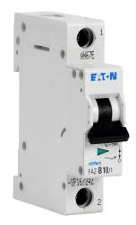
Eaton miniature supplementary protector, 10A, 277 VAC / 48 VDC, 1-pole, B curve, thermal magnetic, 10kA @ 277 VAC interrupting rating, 35mm DIN rail mount.
