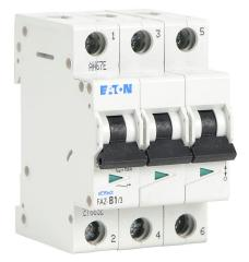
Eaton miniature supplementary protector, 1A, 480Y / 277 VAC / 96 VDC, 3-pole, B curve, thermal magnetic, 10kA @ 480Y/277 VAC interrupting rating, 35mm DIN rail mount.
